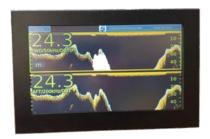
The SKIPPER ESN200 is a dual channel navigation Echo Sounder. The user friendly touch display is intuitive and easy to operate. Most settings may be tuned automatically such as Gain, TVG, Range and Power. The SKIPPER ESN200 is INS and IBS ready as one of the only Echo Sounders in the Market!
